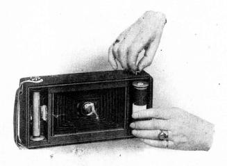
two chambers or receptacles to hold the spools, namely, the film spool and winding spool.
